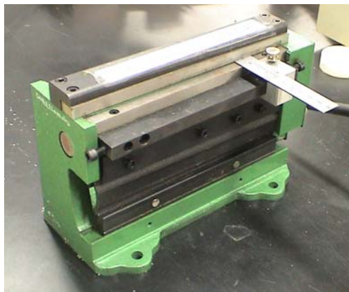
Figure 4.2: Shear for cutting brass cantilever strips for use in stress measurements.
